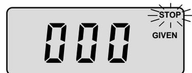
This completes the programming of the CADD-PLUS® pump for Intermittent delivery mode. To verify that you have programmed the values for each mode correctly, press and release the SELECT MODE key to review each value.
